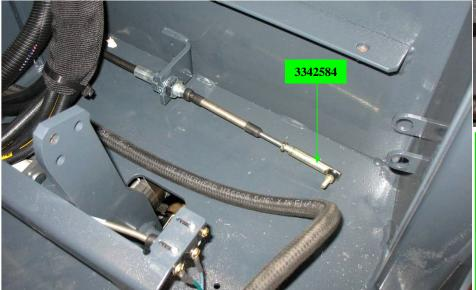
Thread (1) BALL JOINT 1/4-28 LONG LG **3342584** onto end of rod on end of directional cable, as shown above. Tighten.
