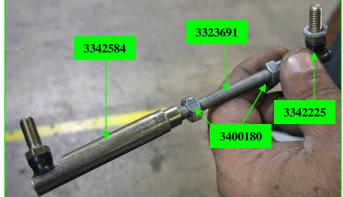
Thread (2) NUT-HEX 1/4-28 ZP **3400180** onto (1) ROD-THREADED 1/4-28 X 2.5 LG **3323691**.
