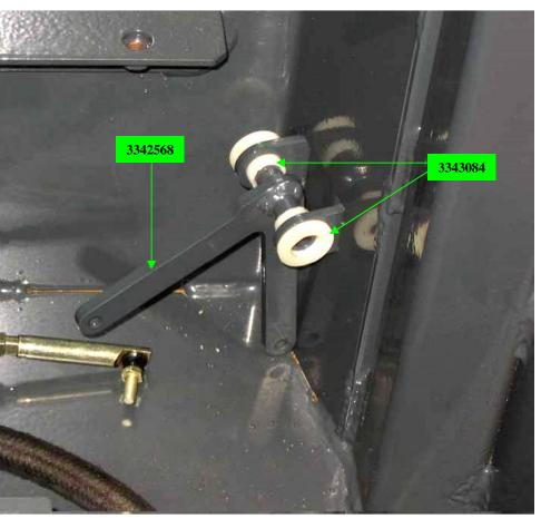
Align WELD-LEVER FWD/AFT CABLE **3342568** with welded bracket in right-front corner of floor of driver's compartment and insert (2) BUSHING-FLING 17/32, NYLON **3343084** through holes to mount WELD-LEVER FWD/AFT CABLE, as shown at right.
