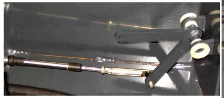
Get (1) SCR-HEX,5/16-18X3.00 GR 5 (**3400467**), (1) NUT-HEX NYLOC 5/16-18 SS (**712683**) and (2) WASHER-FLAT 5/16 ID X .688 OD (**3400088**). Put flat-washer on SCR-HEX,5/16-18X3.00 GR 5 and insert through bushings and WELD-LEVER FWD/AFT CABLE. Secure on back with NUT-HEX NYLOC 5/16-18. Tighten.
